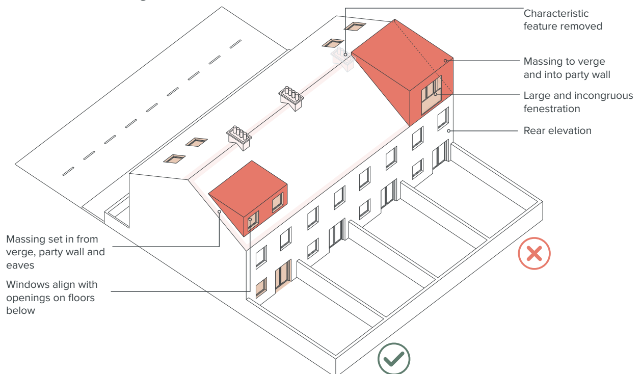
Dormer extensions to terraced houses
